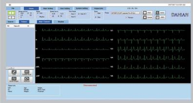
Using ECG Viewer developed by Dahian Pezeshki Pishro Company, ECG data is acquired by connecting YASHAM 310 or YASHAM 110 to PC and in addition to displaying signals on monitor, recording is performed by the printer connected to PC.
